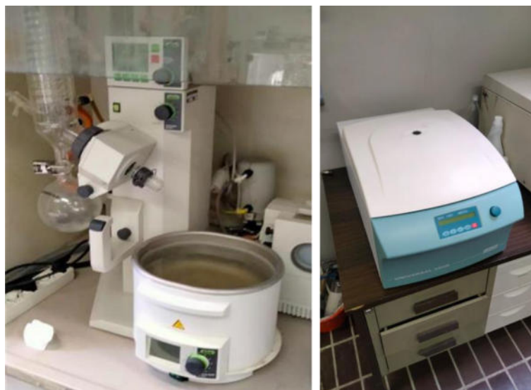
Fig. 6-5. Other equipment used for lipid extraction. Rotavapor BUCHI R-210 on the left, centrifuge UNIVERSAL 320R on the right.
