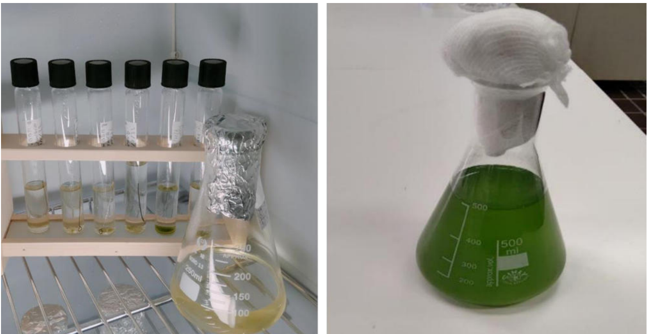
Fig. 6-1. On the left, S. obliquus strains. On the right: solution A flask status after 3% v/v dilution (Solution “A”).
